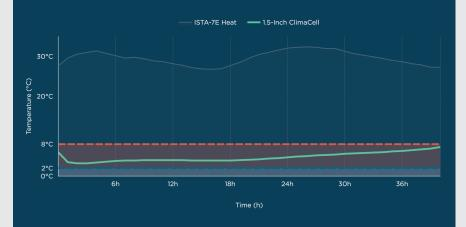
Testing Conditions: 48-hour ISTA-7E Heat thermal test using 11"x9"x12" box dimensions with 2PC with ClimaCell loaded with (3) 24oz frozen gel packs.
